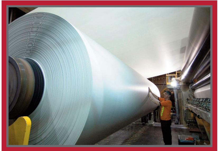
Sheets of paper are wound onto large rolls during the final stages of production at Catalyst's manufacturing plant. Once cut, the rolls are shipped to customers all over the world.
